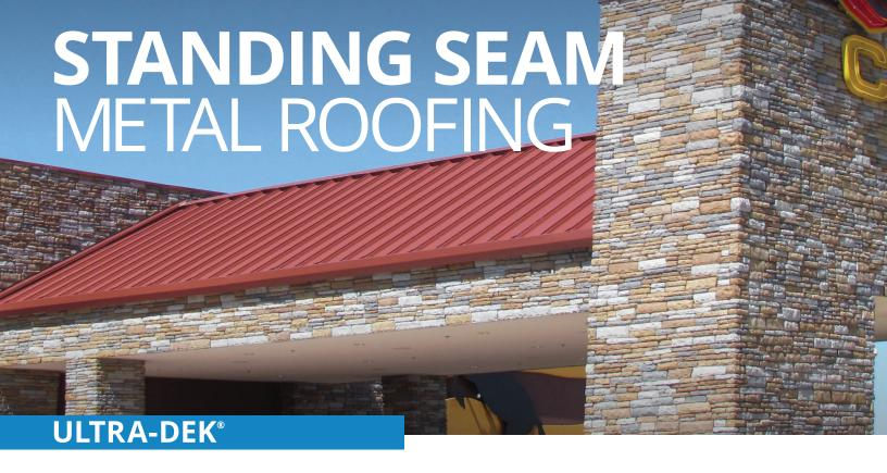
The Ultra-Dek® roof panel is a snap-together, trapezoidal leg standing seam roof system. Ultra-Dek® panels are available in 12-inch, 18-inch and 24-inch widths. Ultra-Dek® requires a minimum slope of 1/2 and is ideal for industrial, commercial and architectural applications. Ultra-Dek® can be erected on various types of construction.
