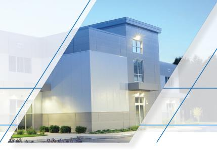
The Metl-Span CF Santa Fe panel has a flat exterior profile with a heavy, embossed stucco texture that mimics the look of a masonry stucco finish but with the added value of an insulated metal panel. The profile is flush with the warmness of an old-world finish, providing a visually pleasing building.
